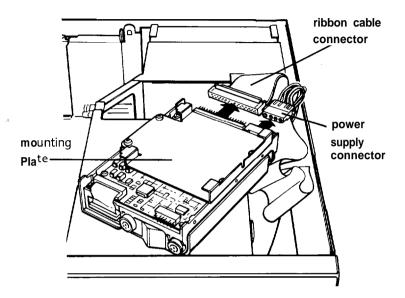
5. Remove the ribbon cable connector from the back of the drive in the same manner, as shown above.
